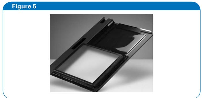
Figure 5: Radiographic phosphor screen installed in the In-Vivo Xtreme II Animal Management Center (AMC) frame. (The AMC is shown outside the In-Vivo Xtreme II cabinet). The open imaging window is shown to the left. The radiographic screen is shown to the right in the inactive position.
