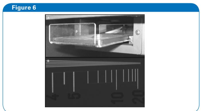
Figure 6: (A) Geometric magnification stage providing X-ray magnification for specimen imaging. (B) Line-pair gauge imaged using X-ray with the In-Vivo Xtreme II.
