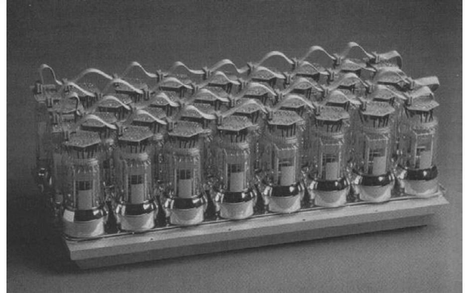
Anger camera (Nal-scintillator and photo multipliers)
